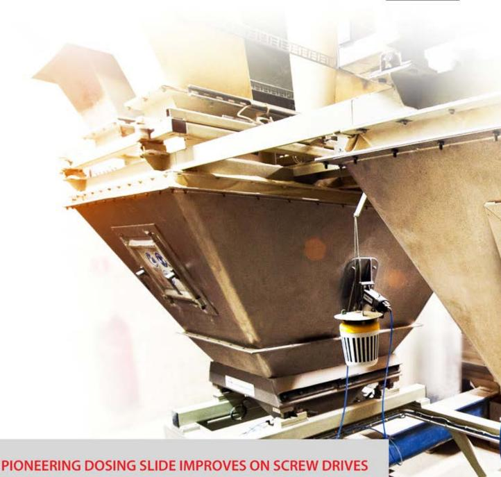
KSE's pioneering dosing slide makes fundamental improvements over traditional dosing systems using screw drives. It has few moving parts for easy maintenance and long life (>20 years). It delivers raw materials with greater speed and accuracy, and has an enormous dynamic flow range (1:1000 !!!).
