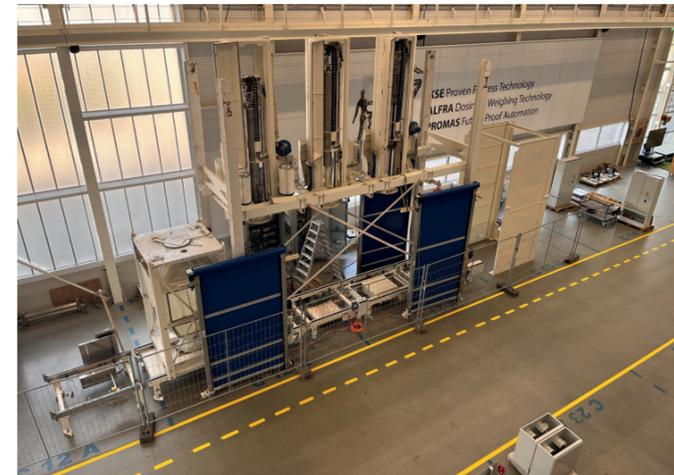
The cleaning system, Clean-in-Place (CIP), is designed to clean and disinfect the dosing containers located on top of the movable dosing machine for medium and small components.
